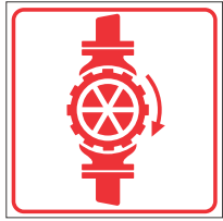
Sprinkler Stop Valve
