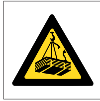
Suspended Loads Hazard
