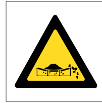
Materials Falling From Conveyor Hazard
