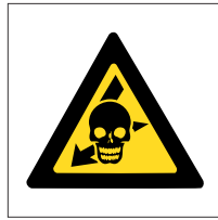
Exposed Live High- Voltage Equipment
